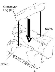
Figure 37 - Installing Crossover Log
